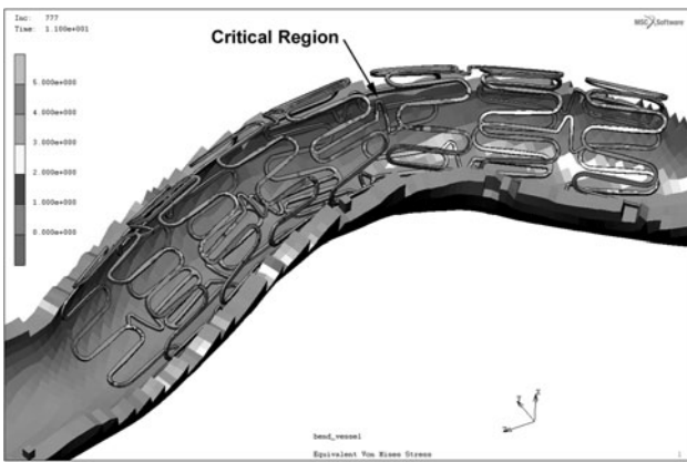
Fig. 14 Nonhelical stent with safety factors contoured from 32° bending fatigue loading
